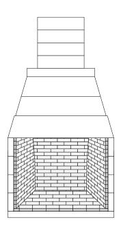
FULLY BRICKED FIREBOX COVERING EXPANSION GAPS
