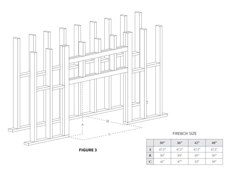
The numbers listed are the framing dimensions recommended by FireRock, which add  $\frac{1}{2}$ " of air space to the required clearances. Always maintain the stated minimum clearance to combustibles for this unit.
