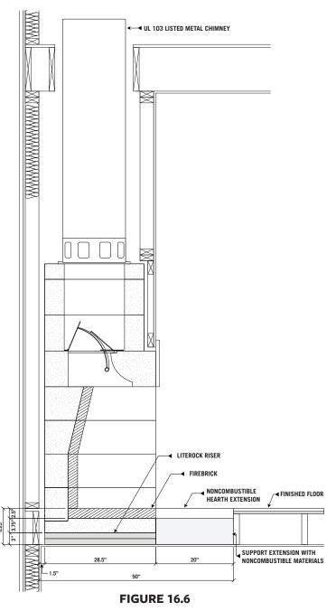
**IMPORTANT:** When installing the LiteRock Riser as a flush hearth application, the noncombustible hearth extension <u>must</u> be supported by noncombustible materials (Figure 16.6). All materials that abut the fireplace or riser material <u>must</u> be noncombustible.
